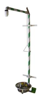
Size Eye and Emergency Shower MB150-30W Article number 99999979 Material Stainless steel bowl, steel tube, plastic shower head Pipework Galvanized Stainless steel push bar and Operation stainless steel pull bar Water flow Eyebath 12 l/min. Emergency shower 80 ltr/min. (2 Bar) 1" BSP internal thread Water supply By means of 2 wall brackets Wall mounting
